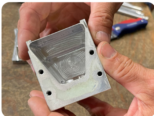
Using OCM makes workpiece machining significantly more efficient and, in most cases, eliminates the need for additional manual rework.
