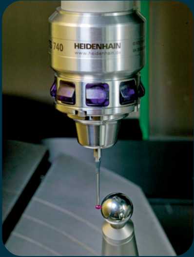
With KinematicsOpt, the machine kinematics are always perfectly calibrated.
