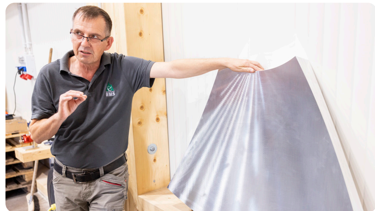
On these high-gloss components, the machine's control performance becomes visible directly on the workpiece surface.
