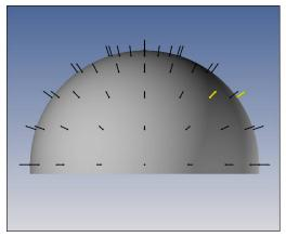
Surface normal vector perpendicular to the contour
